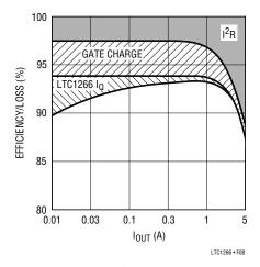
Figure 8. Efficiency Loss
