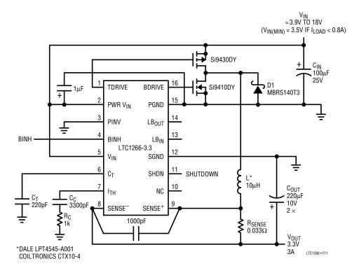
Figure 11. Low Dropout, 3.3V/3A High Efficiency Regulator
