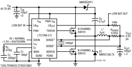
Figure 1. High Efficiency Step-Down Converter
