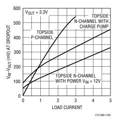
Figure 5. Comparison of Dropout Performance
