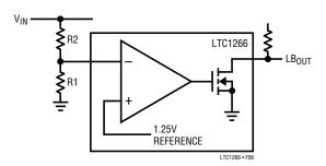
Figure 6. Low-Battery Comparator
