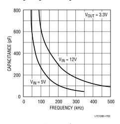
Figure 3. Timing Capacitor Value
