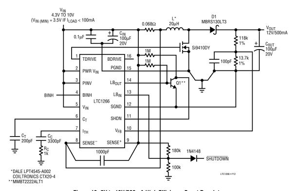
Figure 12. 5V to 12V/500mA High Efficiency Boost Regulator
