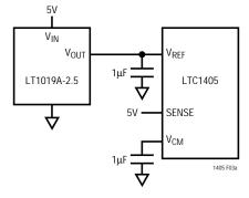
Figure 3a. Using the LT1019-2.5 As an External Reference; Input Range = ±1.25V
