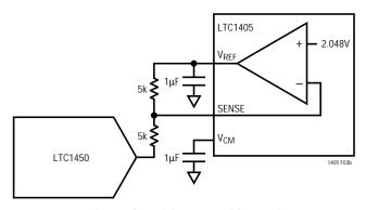
Figure 3b. Driving V<sub>REF</sub> with a DAC
