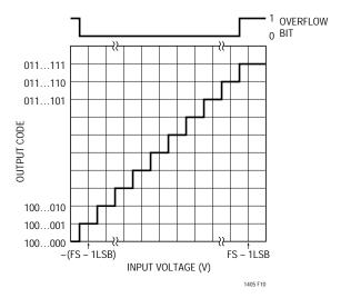
Figure 10. LTC1405 Transfer Characteristics
