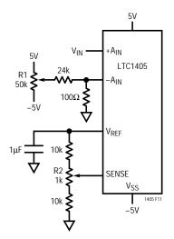
Figure 11. Offset and Full-Scale Adjust Circuit
