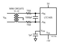
Figure 8b. Dual Supply Transformer Coupled Input
