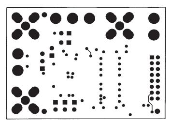
Figure 19. Bottom Layer for LTC1405/LTC1420 Demo Board
