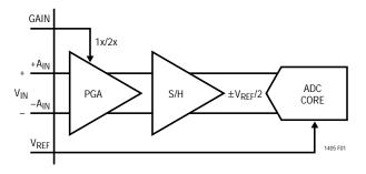
Figure 1. Analog Input Circuit
