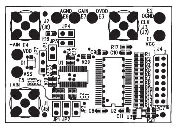
Figure 15. Top Silkscreen Layer for LTC1405/LTC1420 Demo Board
