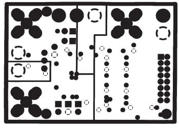
Figure 18. Power Plane Layer for LTC1405/LTC1420 Demo Board
