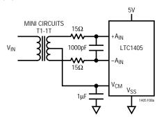
Figure 8a. Single Supply Transformer Coupled Input
