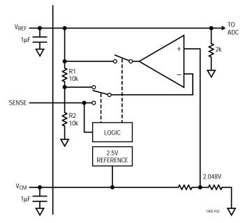
Figure 2. Reference Circuit
