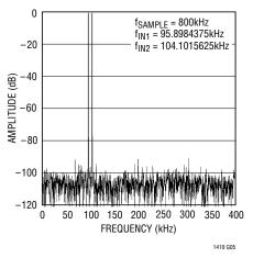
Figure 5. Intermodulation Distortion Plot
