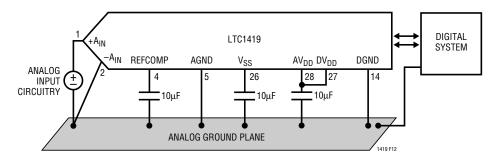
Figure 12. Power Supply Grounding Practice
