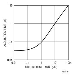
Figure 6. t<sub>ACQ</sub> vs Source Resistance
