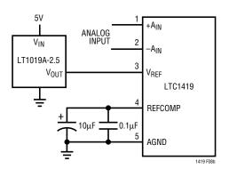
Figure 8b. Using the LT1019-2.5 as an External Reference
