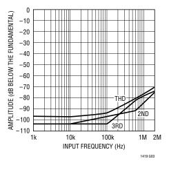
Figure 4. Distortion vs Input Frequency
