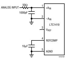
Figure 7. RC Input Filter
