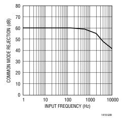
Figure 10a. CMRR vs Input Frequency
