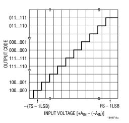
Figure 11a. LTC1419 Transfer Characteristics
