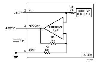
Figure 8a. LTC1419 Reference Circuit
