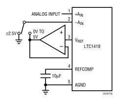
Figure 10b. Selectable OV to 5V or  $\pm 2.5V$  Input Range
