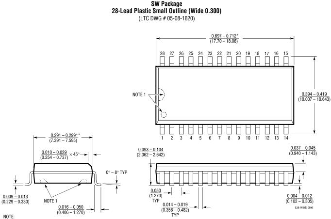
1. PIN 1 IDENT, NOTCH ON TOP AND CAVITIES ON THE BOTTOM OF PACKAGES ARE MANUFACTURING OPTIONS. THE PART MAY BE SUPPLIED WITH OR WITHOUT ANY OF THE OPTIONS
