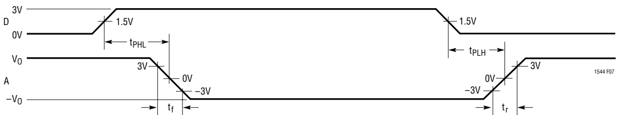
Figure 7. V.10, V.28 Driver Propagation Delays
