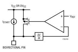
Figure 1. Dynamic Pull-Up Current Sources
