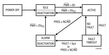
Figure 4. LTC1755 State Diagram
