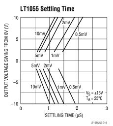
LT1056 Settling Time 10 OUTPUT VOLTAGE SWING FROM 0V (V) 10m\ 2mV 0.5mV 5 5mV 1mV  $V_S = \pm 15V$  $T_A = 25^{\circ}C$ 0 5mV -5 10m\ 2mV 1mV 0.5mV -10 0 2 3 1 SETTLING TIME (µS) LT1055/56 G20
