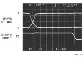
Figure 12. Receiver  $t_{PLH}$
