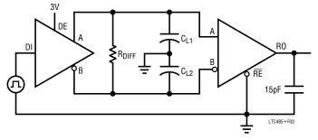
Figure 3. Driver/Receiver Timing Test Circuit
