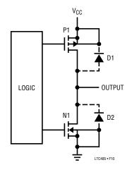
Figure 10. Conventional CMOS Output Stage
