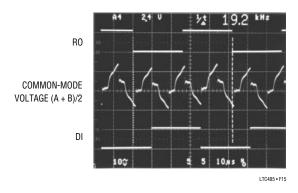
Figure 15. System Common-Mode Voltage at 19.2kHz
