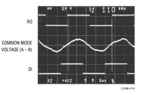
Figure 18. System Differential Voltage at 110kHz
