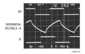
Figure 16. System Differential Voltage at 19.2kHz
