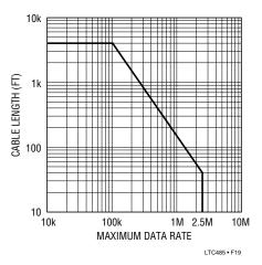
Figure 19. Cable Length vs Maximum Data Rate
