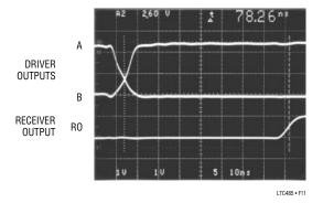
Figure 11. Receiver t<sub>PHL</sub>
