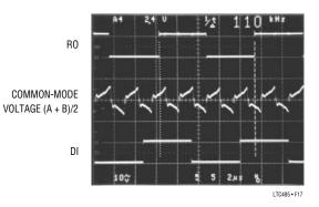
Figure 17. System Common-Mode Voltage at 110kHz
