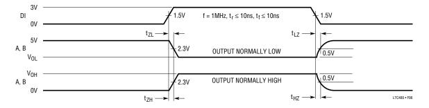
Figure 6. Driver Enable and Disable Times
