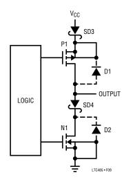
Figure 9. LTC485 Output Stage
