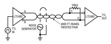
Figure 14. Line Length Test Circuit
