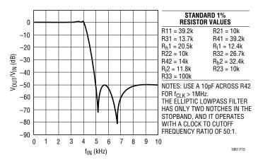
Figure 15. Resistor Values and Amplitude Response of the Topology of Figure 12.
