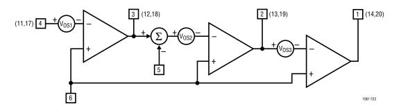
Figure 23. Equivalent Input Offsets of 1/3 LTC1061 Filter Building Block.
