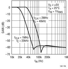
Figure 6. Measures Frequency Response of the Lowpass Butterworth Filter of Figure 3.
