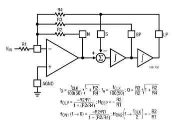
Figure 20. Mode 2: 2nd Order Filter Providing Notch, Bandpass, Lowpass.
