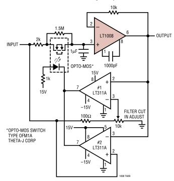
This circuit is useful where fast signal acquisition and high precision are required, as in electronic scales.
