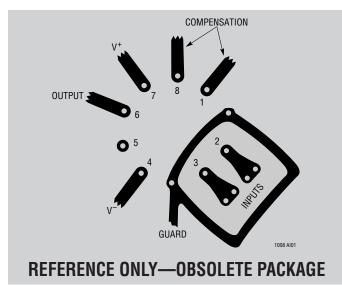
Microvolt level error voltages can also be generated in the external circuitry. Thermocouple effects caused by temperature gradients across dissimilar metals at the contacts to the input terminals can exceed the inherent drift of the amplifier. Air currents over device leads should be minimized, package leads should be short, and the two input leads should be as close together as possible and maintained at the same temperature.
