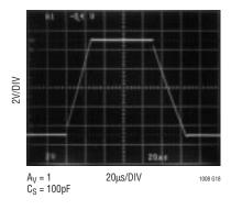
Slew Rate vs Compensation Capacitance
