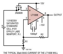
THE TYPICAL 30pA BIAS CURRENT OF THE LT1008 WILL DEGRADE THE STANDARD CELL BY ONLY 1ppm/YEAR. NOISE IS A FRACTION OF A ppm. UNPROTECTED GATE MOSFET ISOLATES STANDARD CELL ON POWER DOWN
