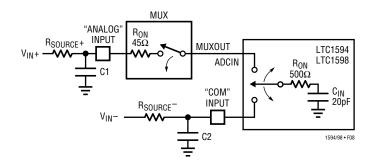
Figure 8. Analog Input Equivalent Circuit
