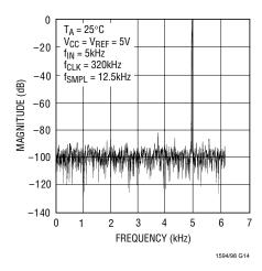
Figure 10. LTC1594/LTC1598 Nonaveraged, 4096 Point FFT Plot
