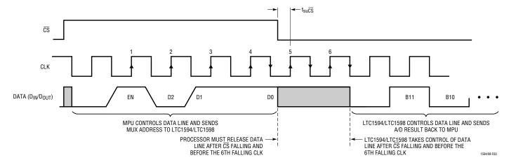
Figure 3. LTC1594/LTC1598 Operation with D<sub>IN</sub> and D<sub>OUT</sub> Tied Together
