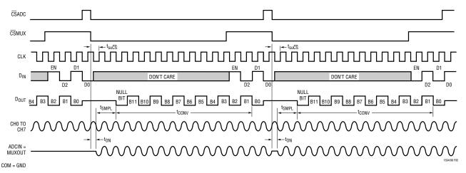
Figure 5. Use Separate Chip Selects to Maximize Sample Rate
