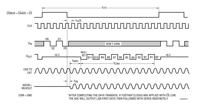
Figure 1. LTC1594/LTC1598 Operating Sequence Example: CH2, GND
