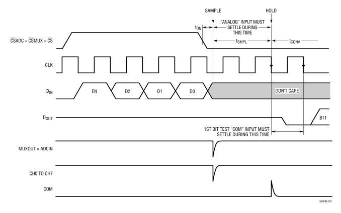
Figure 7. LTC1594/LTC1598 ADCIN and COM Input Settling Windows
