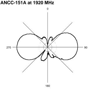
Azimuth Plane is omnidirectional within ± 1.5 dB.
