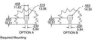
(without bracket) MIN MOUNTING PANE THICKNESS .06 MAX MOUNTING THICKNESS .33
