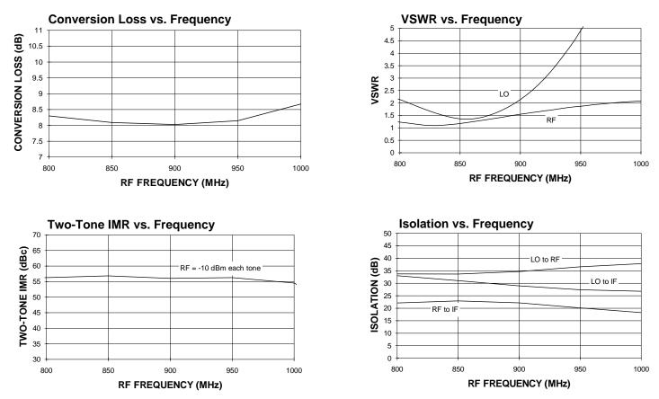
1. Test Conditions for Down Converter Application: RF=900 MHz (-10 dBm), IF=60 MHz, LO=840 MHz (+5 dBm), LO Port match shown on Page 2. 2. Test Conditions for Up Converter Application: LO=840 MHz (+5 dBm), IF=60 MHz (-10 dBm), RF=900 MHz, LO Port match shown on Page 2.
