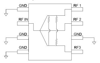
Pins labeled as ground should be DC and RF grounded.
