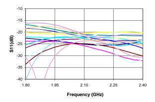
**Output Return Loss vs. Frequency** (+85°C)
