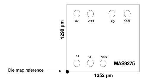
Note 1: MAS9275 pads are round with 80  $\mu m$  diameter at opening.
