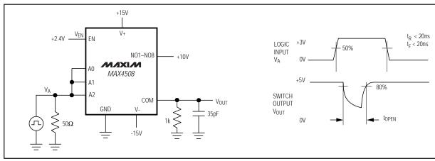
Figure 4. MAX4508 Break-Before-Make Interval
