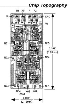
TRANSISTOR COUNT: 543 SUBSTRATE IS INTERNALLY CONNECTED TO V+. MAX4508/MAX4509
