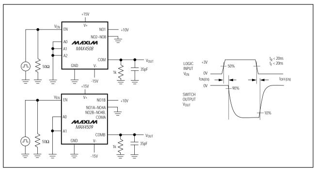
Figure 3. Enable Switching Time
