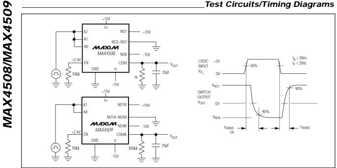
Test Circuits/Timing Diagrams
