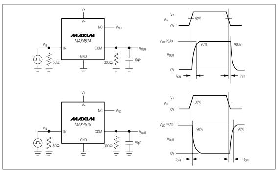
Figure 2. Switching Times
