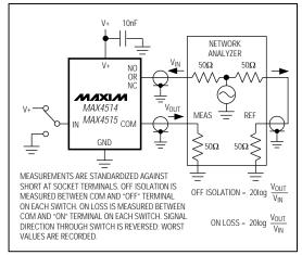
Figure 3. Off Isolation and On Loss
