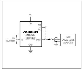
Figure 4. NO, NC, and COM Capacitance
