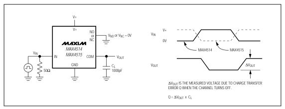
Figure 1. Charge Injection
