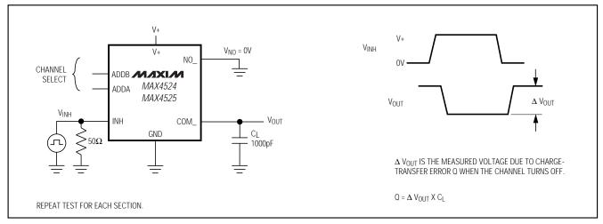
Figure 4. Charge Injection
