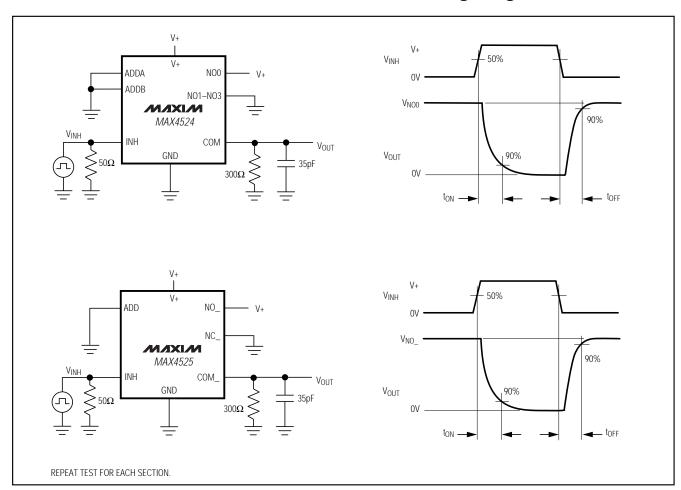
Figure 2. Inhibit Switching Times
