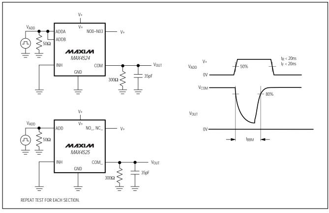
Figure 3. Break-Before-Make Interval
