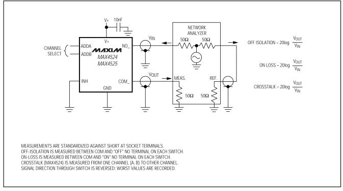
Figure 5. Off-Isolation, On-Loss, and Crosstalk
