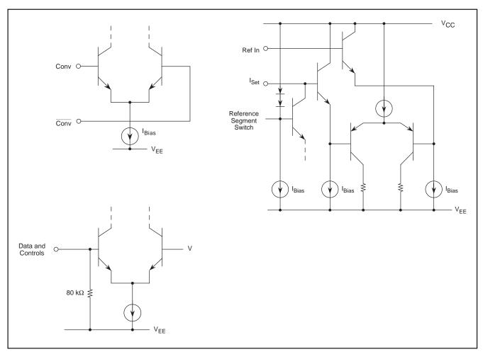
Figure 2. Equivalent Input Circuits—Data, Clock, Controls, and Reference
