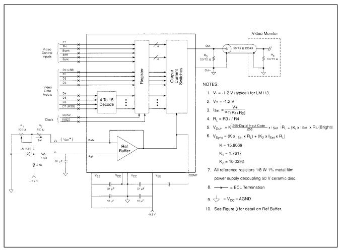
Figure 1. Typical Interface Circuit
