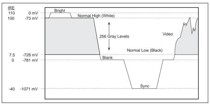
Figure 5. Video-Output Waveform for Standard Load
