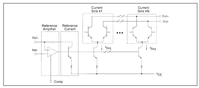
Figure 3. Reference Buffer and DAC Output Circuit
