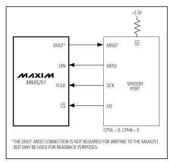
Figure 3. Connections for SPI/QSPI
