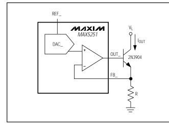
Figure 13. Digitally Programmable Current Source
