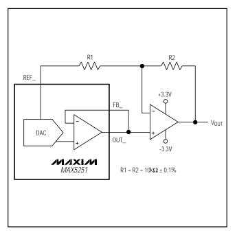
Figure 11. Bipolar Output Circuit
