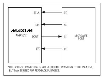
Figure 2. Connections for Microwire
