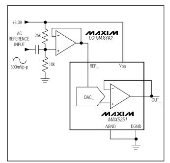
Figure 12. AC Reference Input Circuit
