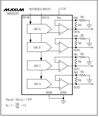
Figure 10. Unipolar Rail-to-Rail Output Circuit
