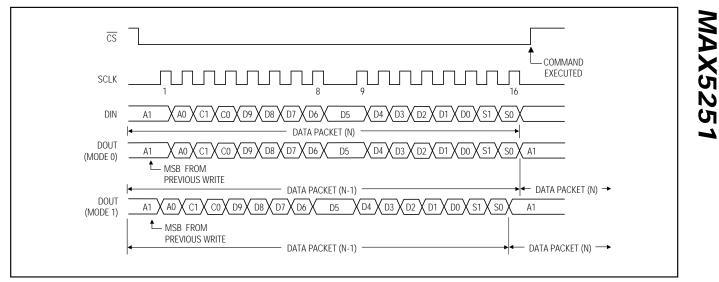
Figure 5. Serial-Interface Timing Diagram
