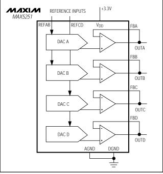
Figure 9. Unipolar Output Circuit
