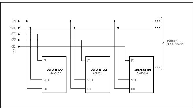
Figure 8. Multiple MAX5251s Sharing a Common DIN Line
