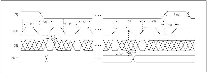
Figure 6. Detailed Serial-Interface Timing Diagram
