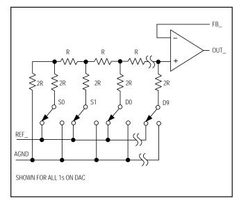
Figure 1. Simplified DAC Circuit Diagram
