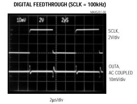
$\overline{\text{CS}} = \overline{\text{PDL}} = \overline{\text{CL}} = 3.3\text{V}, \text{ DIN} = 0\text{V}$ DAC A CODE SET TO 800 hex
