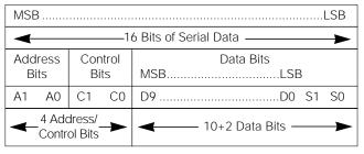
Figure 4. Serial-Data Format
