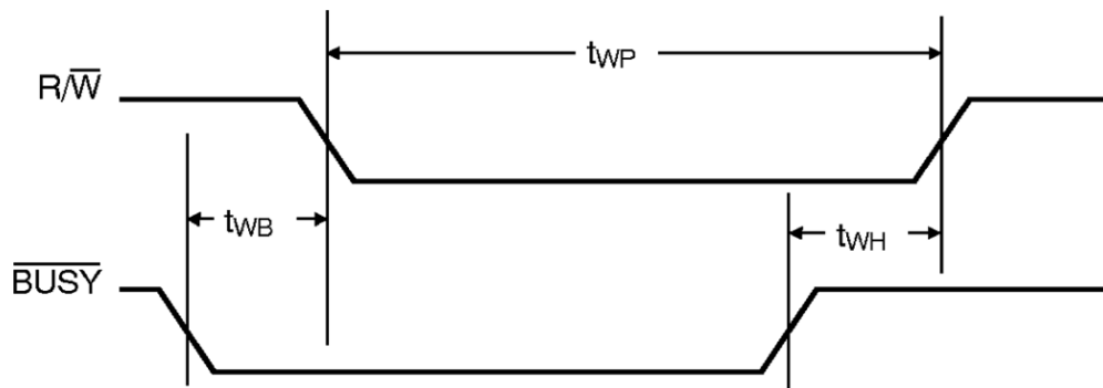
FIGURE 8. TIMING WAVEFORM OF WRITE WITH \overline{BUSY} (FOR SLAVE)
