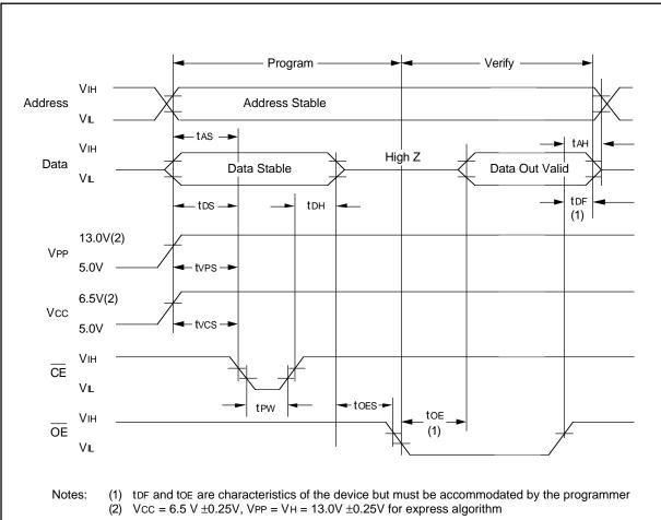
FIGURE 1-2: PROGRAMMING WAVEFORMS
