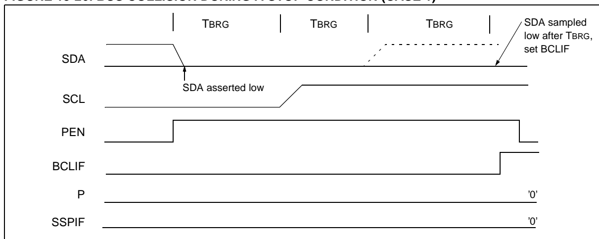
FIGURE 15-26: BUS COLLISION DURING A STOP CONDITION (CASE 1)
