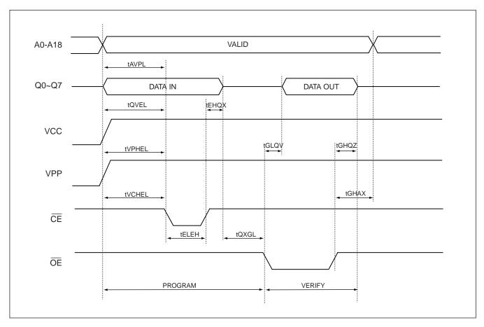
Table 3. Programming Mode AC Characteristics <sup>(1)</sup> (TA=25℃; VCC=6.25V±0.25V; VPP=12.5V±0.25V)
