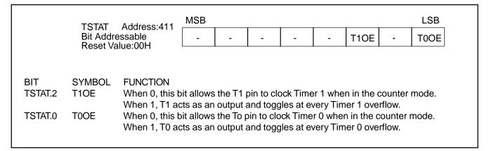
Figure 9. Timer 0 and 1 Extended Status (TSTAT)
