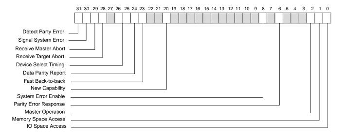
The bit content will be reset to 0 when a 1 is written to the corresponding bit location.
