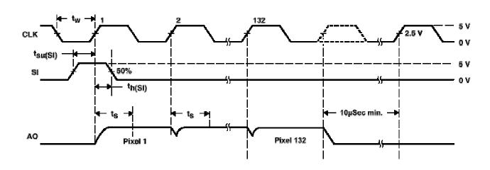
All tests are made with 3.5ms integration time, at  $10\mu$ W/cm<sup>2</sup> light = 100% at 25°C at 880 nm and with a clock speed of 500kHz in, and 250kHz out, unless otherwise specified in the Test Conditions.
