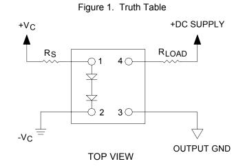
Figure 2. Terminal Connections
