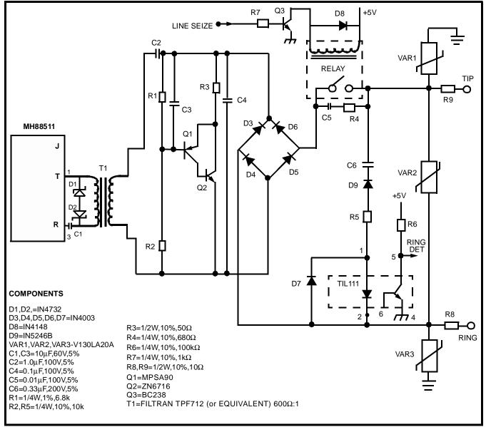
Figure 7 - MH88511 as a Trunk Interface Application
