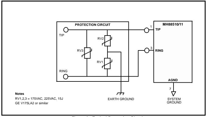
Figure 6 - Typical Protection Circuit
