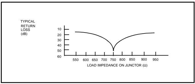
Figure 4 - Return Loss VS Junctor Load Impedance
