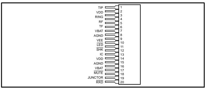
Figure 2 - Pin Connections
