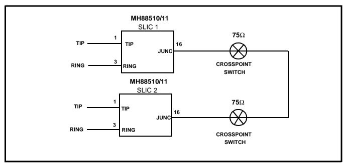
Figure 3 - SLIC Crosspoint Switch Connection
