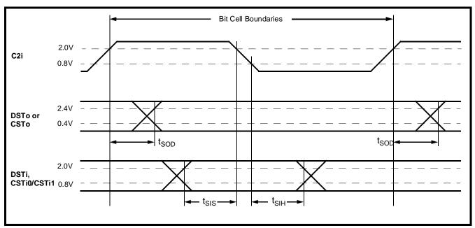
Figure 15 - ST-BUS Stream Timing
