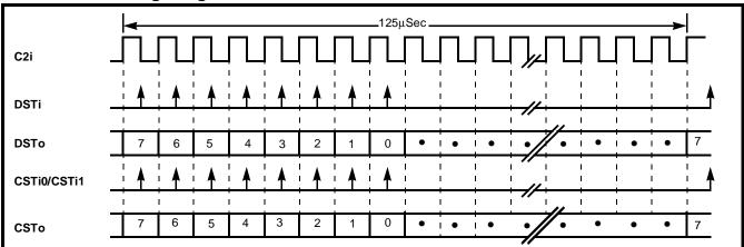
Figure 3 - ST-BUS Timing
