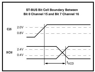
Figure 16 - XCtl Timing
