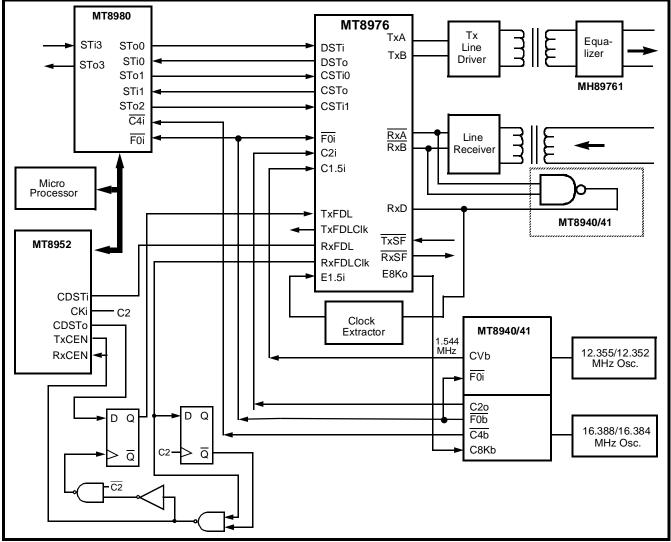
Figure 10 - Typical ESF Configuration
