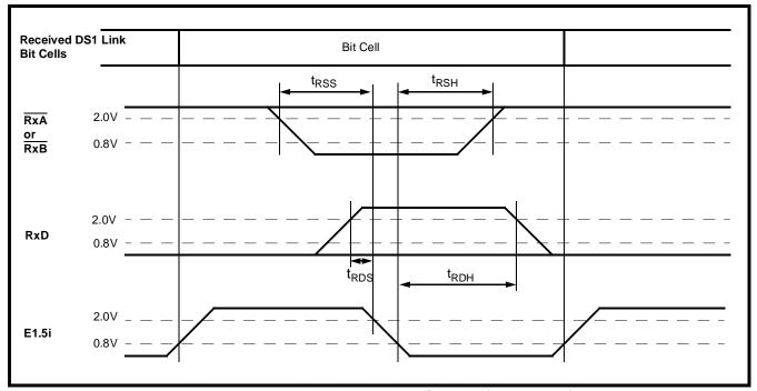
Figure 20 - Receive Timing for DS1 Link (see Note 1)
