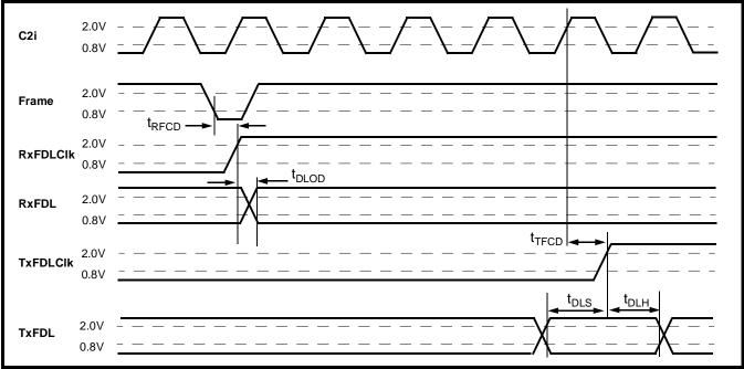
Figure 22 - Facility Data Link Timing
