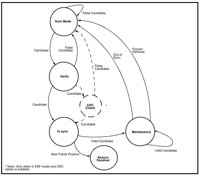
Figure 8 - Off-Line Framer State Diagram
