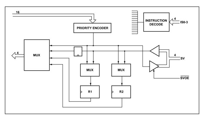
Fig.3 Shift control block
