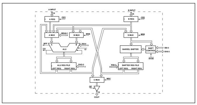
Fig.2 PDSP1601 block diagram
