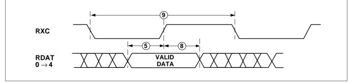
Fig.5 Receive timing waveform
