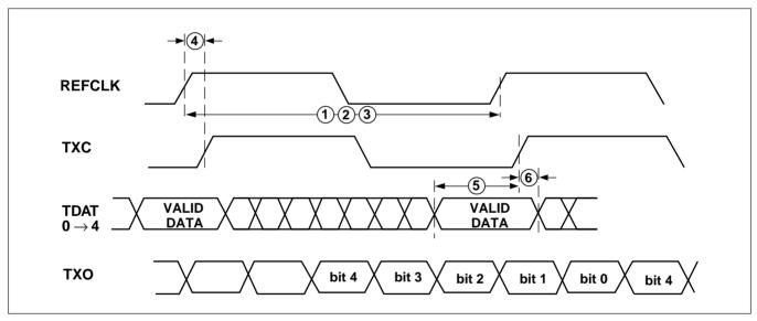
Fig.4 Transmit timing waveform
