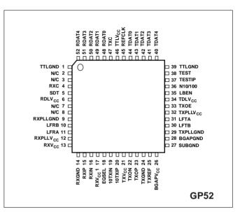
Fig.1 Pin connections - top view
