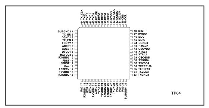
Figure 2Pin connections
