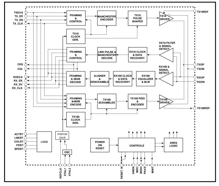
Figure 6 NWK933 block diagram
