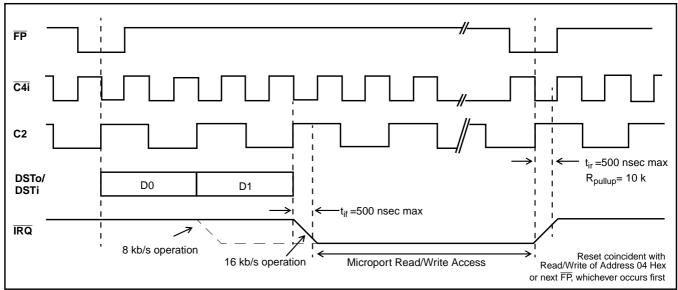
Figure 7b - IRQ Timing Diagram
