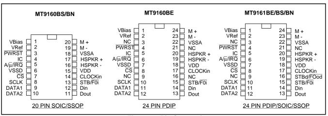
Figure 2 - Pin Connections
