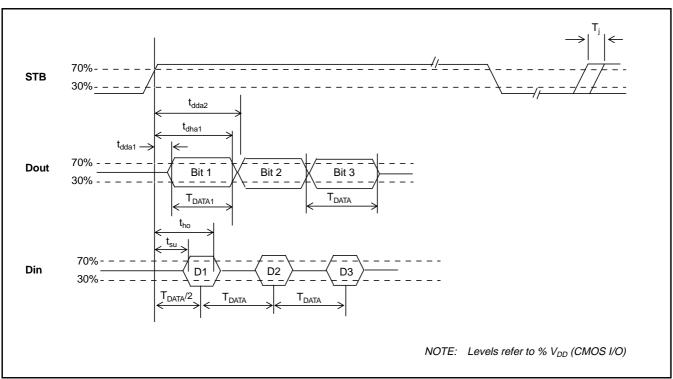
Figure 13 - SSI Asynchronous Timing Diagram
