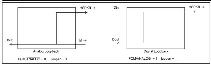
Figure 8 - Loopback Signal Flows
