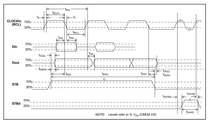
Figure 12 - SSI Synchronous Timing Diagram
