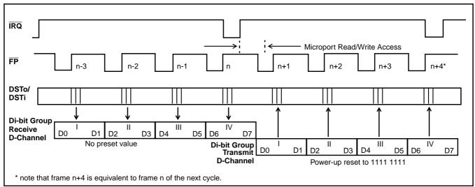
Figure 7a - D-Channel 16 kb/s Operation
