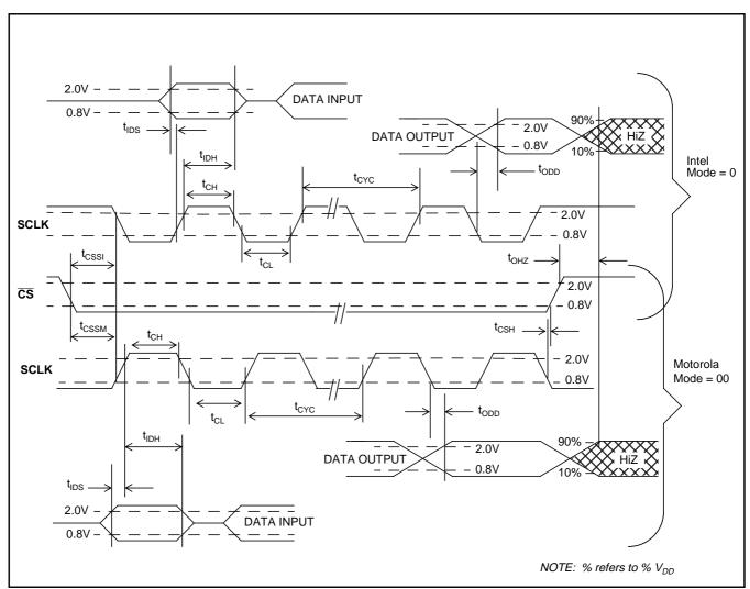
Figure 14 - Microport Timing
