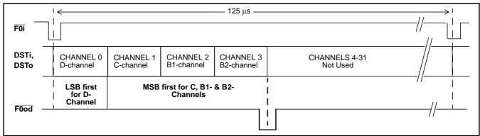
Figure 6 - ST-BUS Channel Assignment
