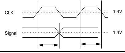
Any AC timing is referenced to the input signal passing through 1.4V.
