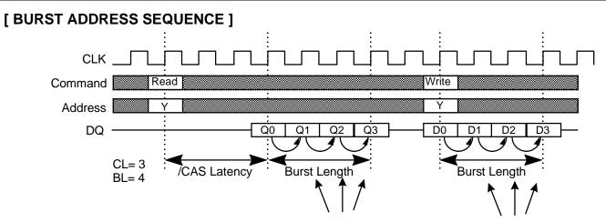
Internal addresses are determined by Burst Type.
