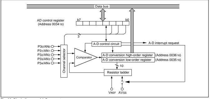
Fig. 38 Block diagram of A-D converter
