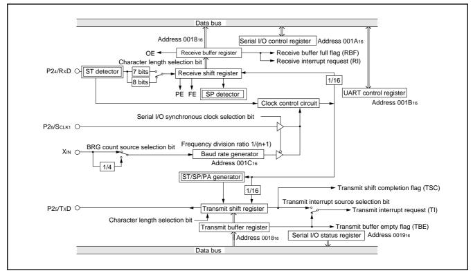
Fig.16 Block diagram of UART serial I/O
