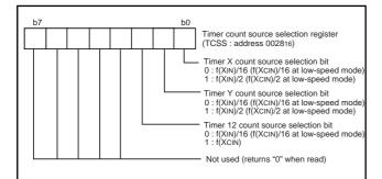
Fig. 12 Structure of timer count source selection register
