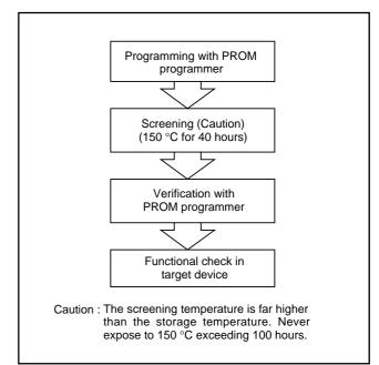
Fig. 49 Programming and testing of One Time PROM version
