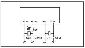
Fig. 44 Ceramic resonator circuit
