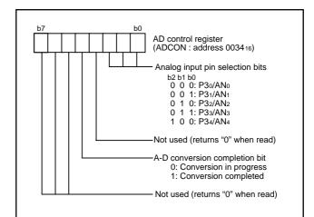
Fig. 36 Structure of AD control register
