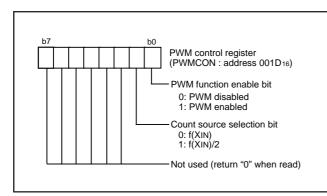
Fig. 34 Structure of PWM control register
