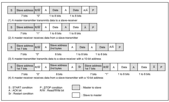
Fig. 31 Address data communication format
