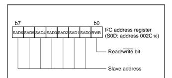
Fig. 20 Structure of I<sup>2</sup>C address register
