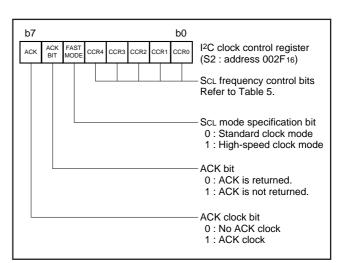
Fig. 21 Structure of I<sup>2</sup>C clock control register
