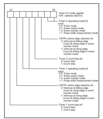
Fig. 11 Structure of timer XY mode register
