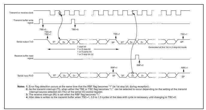
Fig. 17 Operation of UART serial I/O function
