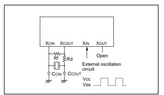
Fig. 45 External clock input circuit
