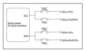
Fig. 22 SDA/SCL pin selection bit
