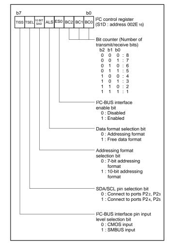
Fig. 23 Structure of I<sup>2</sup>C control register
