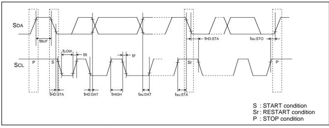
Fig. 53 Timing diagram of multi-master I<sup>2</sup>C-BUS
