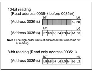
Fig. 37 Structure of A-D conversion registers
