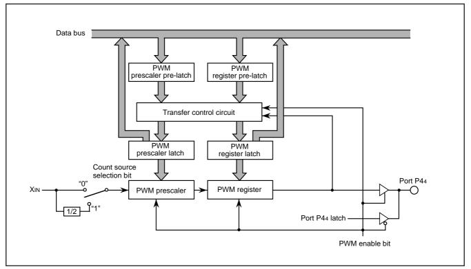
Fig. 33 Block diagram of PWM function
