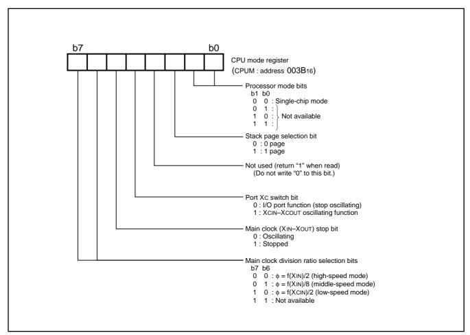
Fig. 4 Structure of CPU mode register
