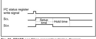
Fig. 26 START condition generating timing diagram
