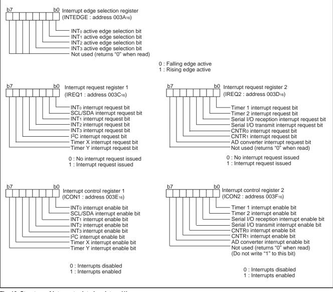
Fig. 10 Structure of interrupt-related registers (1)
