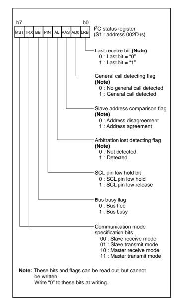
Fig. 24 Structure of I<sup>2</sup>C status register
