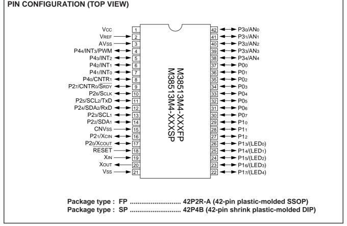
Fig. 1 M38513M4-XXXFP/SP pin configuration
