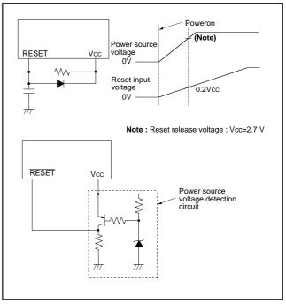
Fig. 41 Reset circuit example
