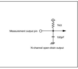
Fig. 51 Circuit for measuring output switching characteristics (2)
