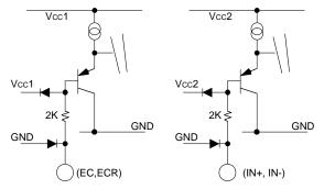
(4)HB output terminal equivalent circuit
