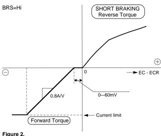
is shown in Figure 1,2 and 3. The current gain is 0.8A/V(at sensing resistor:0.5ohm) in forward torque directions, and the dead zone is from0mV to 60mV. When the reverse brake mode(BRS=Lo) is selected, the coil current gain under the reverse torque control is the same with in
