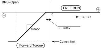
When the free run mode(BRS=open) is selected, the coil current under the reverse torque control (EC-ECR>0) becomes zero and in free run situation.
