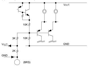
(7)Spindle driver output stage equivalent circuit
