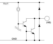
(6)S/S, MUTE, FGS input terminal equivalent circuit
