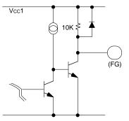
(5)BRS input terminal equivalent circuit
