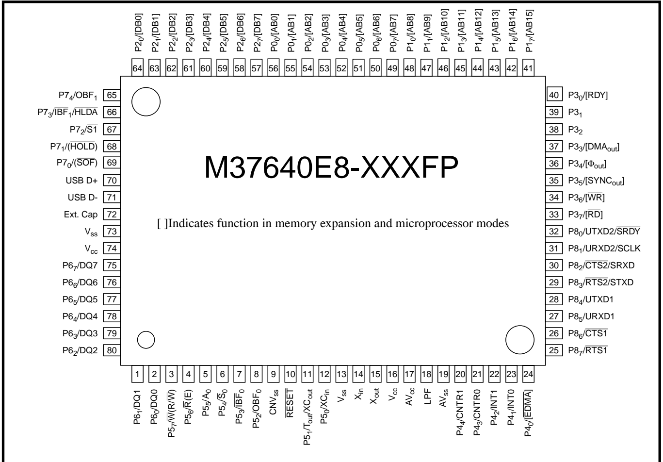
Figure 1-2. Pin Layout
