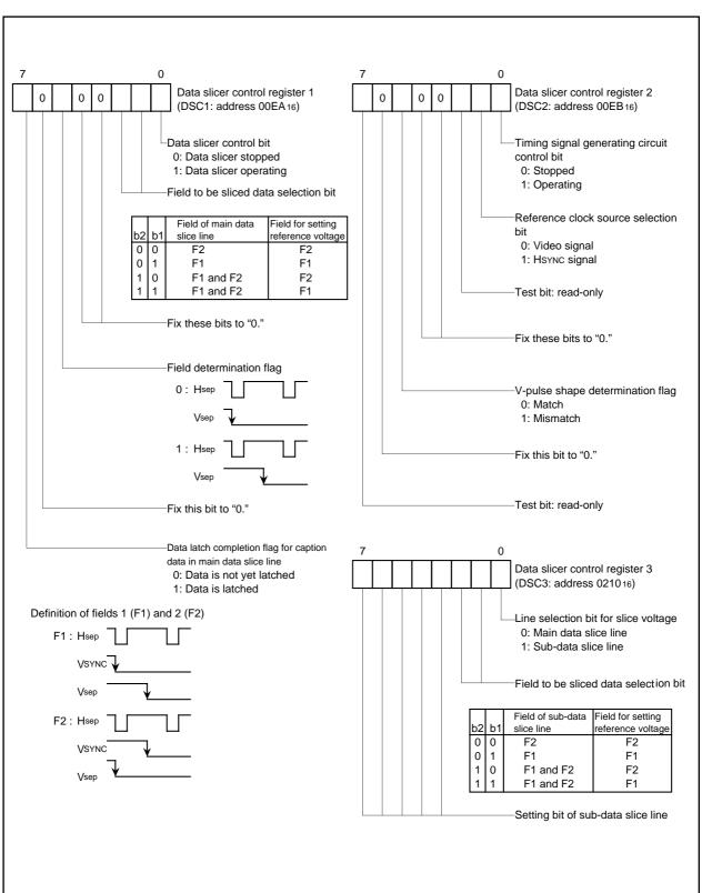
Fig. 26. Data Slicer Control Registers
