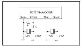
Fig. 95. Ceramic Resonator Circuit Example
