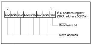
Fig. 43. I<sup>2</sup>C Address Register
