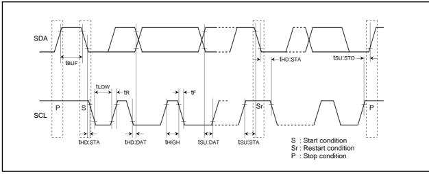
Fig. 101. Definition Diagram of Timing on Multi-master I<sup>2</sup>C-BUS
