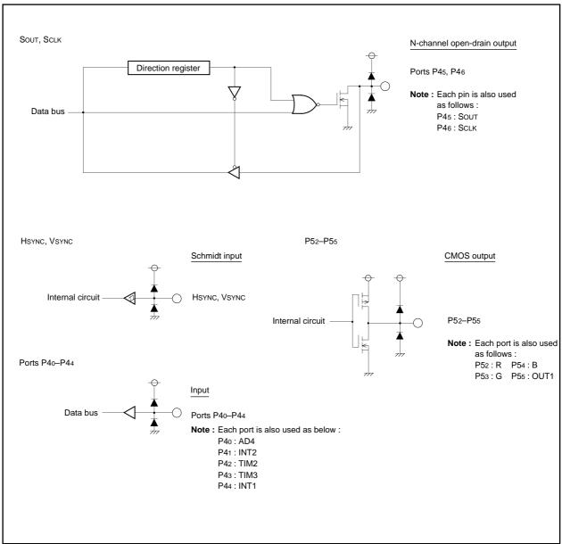
Fig. 2. I/O Pin Block Diagram (2)
