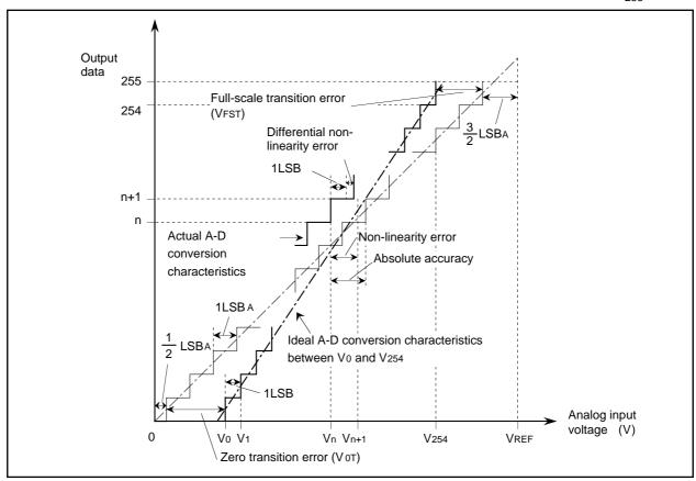
Fig. 24. Definition of A-D Conversion Accuracy
