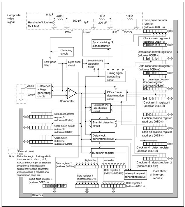
Fig. 25. Data Slicer Block Diagram
