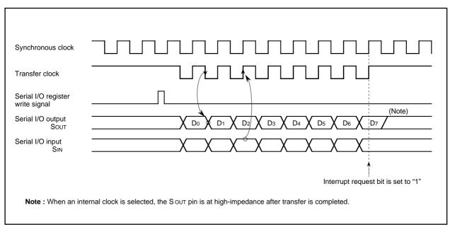
Fig. 15. Serial I/O Timing (for LSB first)
