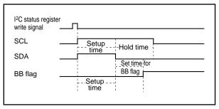
Fig. 49. START Condition Generation Timing Diagram
