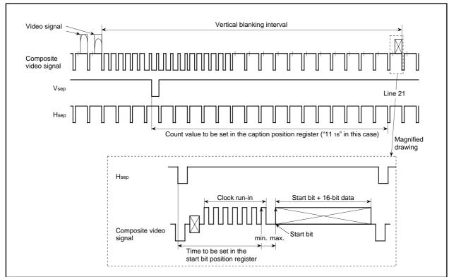
Fig. 30. Signals in Vertical Blanking Interval
