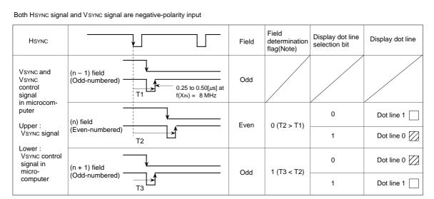
When using the field determination flag, be sure to set bit 0 of the PWM mode register 1 (address 020A 16) to "0."
