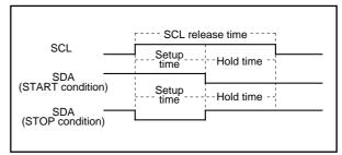
Fig. 51. START Condition/STOP Condition Detect Timing
