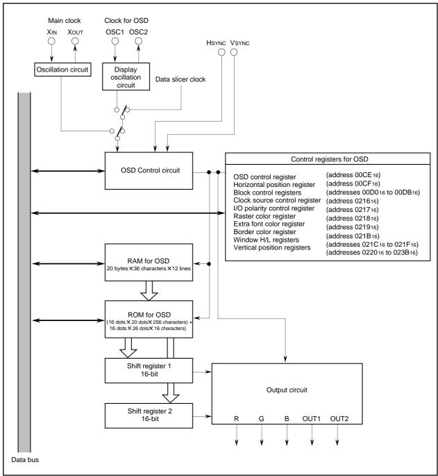
Fig. 54. Block Diagram of OSD Circuit
