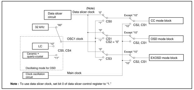
Fig. 67. Block Diagram of OSD Selection Circuit
