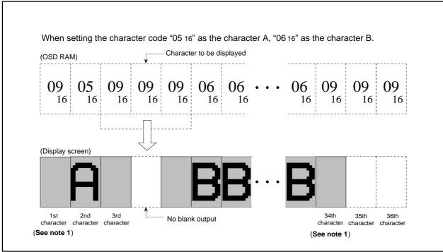
Fig. 84. Display Screen Example of Automatic Solid Space
