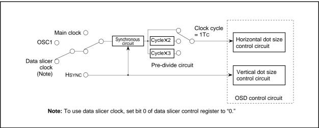
Fig. 64. Block Diagram of Dot Size Control Circuit
