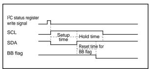
Fig. 50. STOP Condition Generation Timing Diagram
