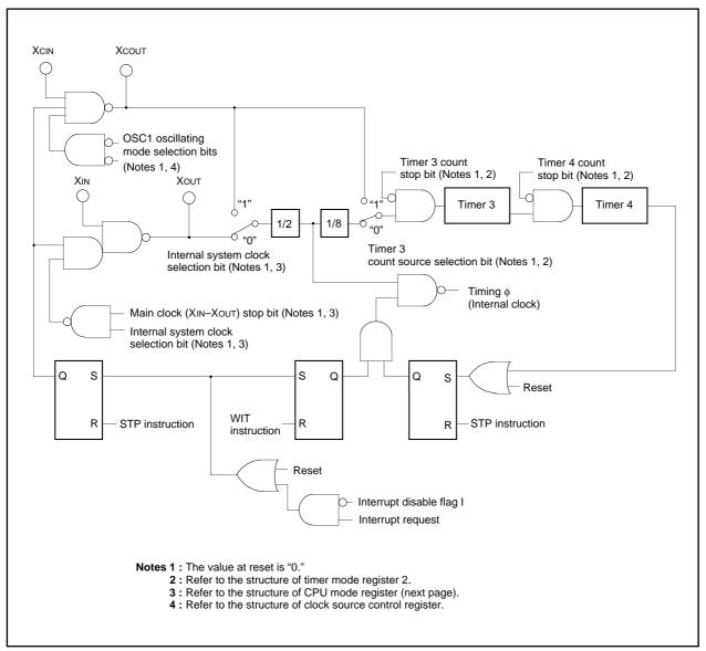
Fig. 97. Clock Generating Circuit Block Diagram
