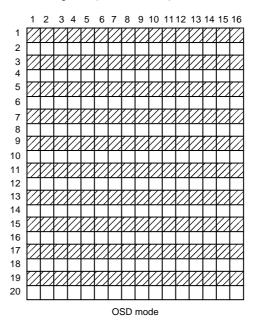
When the display dot line selection bit is "0," the " " " font is displayed at even field, the " " or tis displayed at odd field. Bit 7 of the I/O polarity control register can be read as the field determination flag: "1" is read at odd field, "0" is read at even field.
