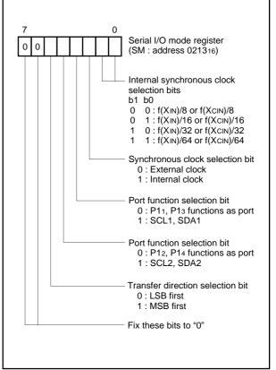
Fig. 16. Serial I/O Mode Register
