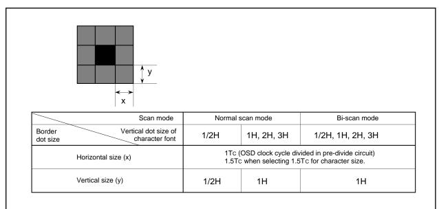
Fig. 79. Horizontal and Vertical Size of Border
