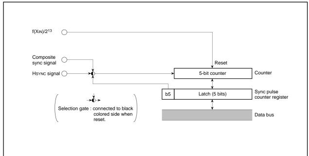
Fig. 41. Synchronous Signal Counter Block Diagram
