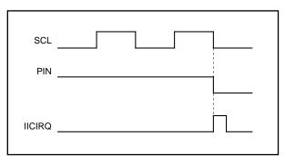
Fig. 48. Interrupt Request Signal Generation Timing
