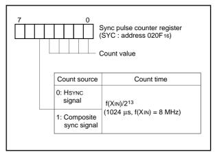
Fig. 40. Sync Pulse Counter Register
