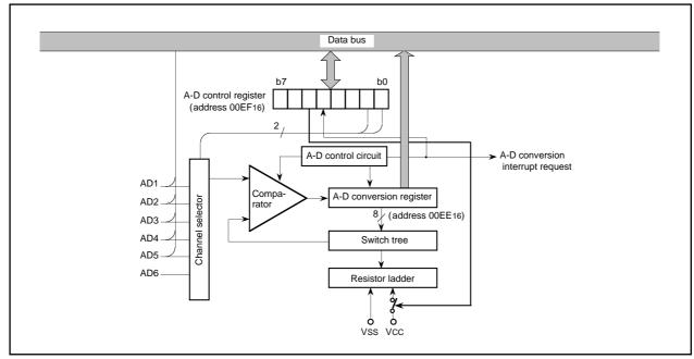
Fig. 22. A-D Comparator Block Diagram
