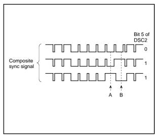
Fig. 29. Determination of V-pulse Waveform
