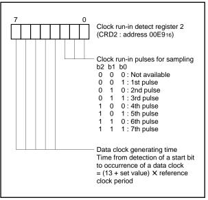
Fig. 34. Clock Run-in Detect Register 2
