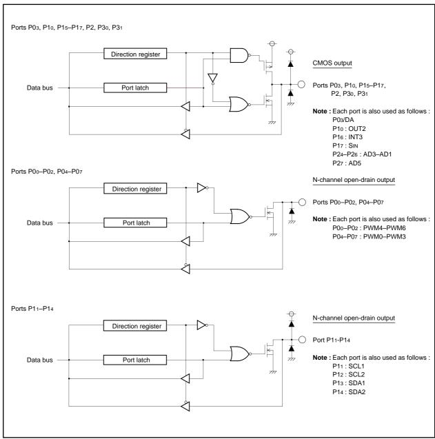
Fig. 1. I/O Pin Block Diagram (1)
