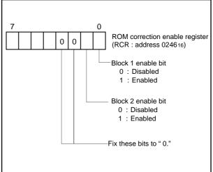
Fig. 92. ROM Correction Enable Register
