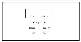
Fig. 99. Display Oscillation Circuit
