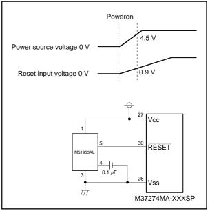
Fig. 93. Example of Reset Circuit
