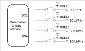
**Note:** When using multi-master I<sup>2</sup>C-BUS interface, set bits 3 and 4 of the serial I/O mode register (address 021316) to "1." Moreover, set the corresponding direction register to "1" to use the port as multi-master I<sup>2</sup>C-BUS interface.
