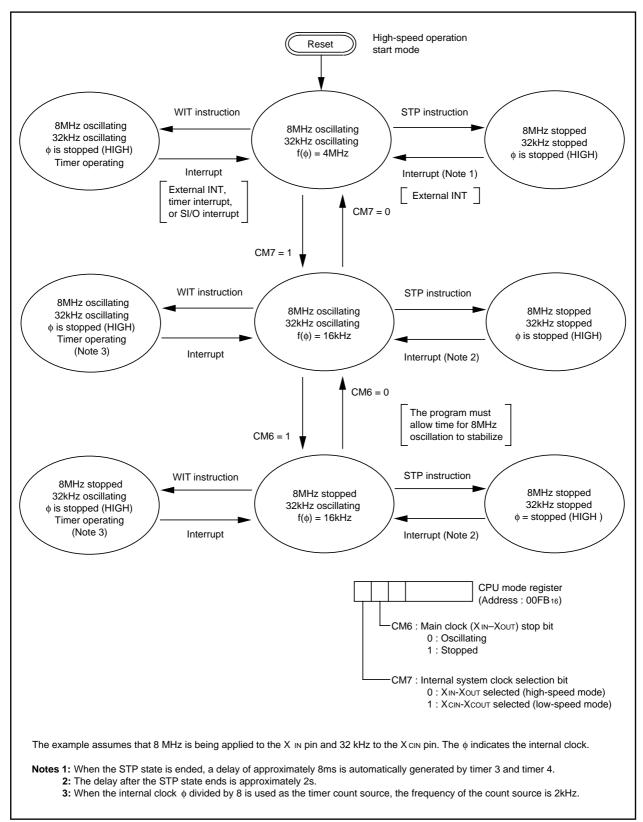
Fig. 98. State Transitions of System Clock
