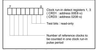
Fig. 39. Clock Run-in Detect Registers 1 and 3
