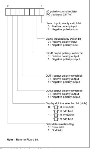
Fig. 68. I/O Polarity Control Register
