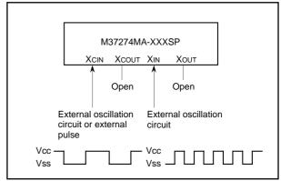
Fig. 96. External Clock Input Circuit Example
