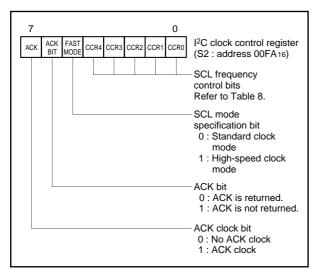
Fig. 44. I<sup>2</sup>C Clock Control Register
