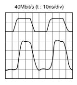
Note: The delay from the DATA input to the laser light output contains the delay occurring in measuring systems.
