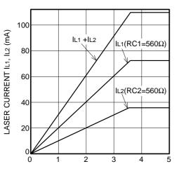
LASER CURRENT VS. CURRENT SETTING VOLTAGE
