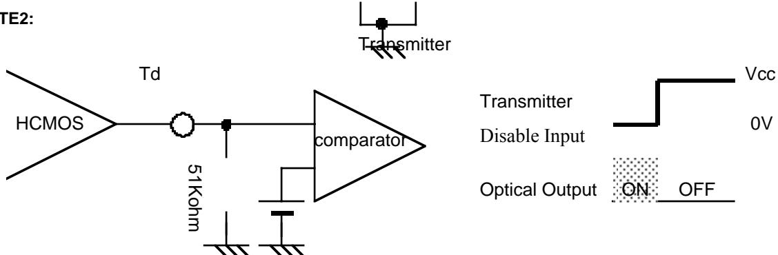
The transmitter is normally enabled and only requires an external voltage to disable.
