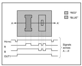
Fig. 47. Example of raster coloring
