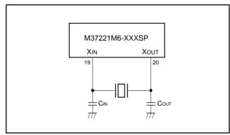
Fig. 54. Ceramic resonator circuit example
