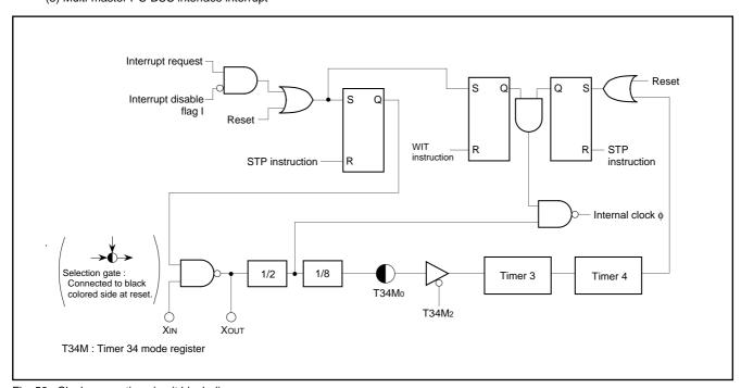
Fig. 56. Clock generating circuit block diagram
