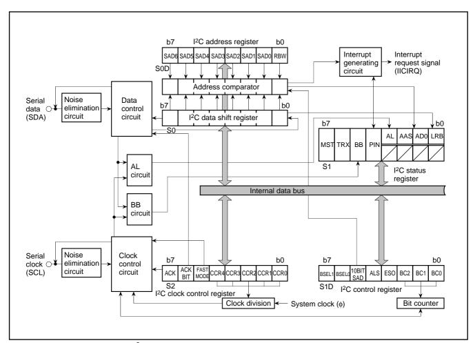
Fig. 12. Block diagram of multimaster I<sup>2</sup>C-BUS interface
