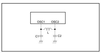
Fig. 57. Display oscillation circuit
