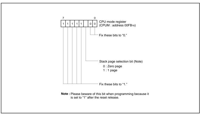
Fig. 1. Structure of CPU mode register
