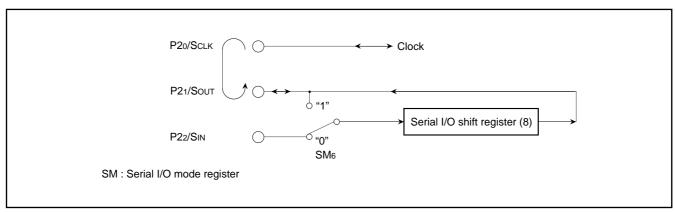
Fig. 11. Signals on serial I/O common transmission/reception mode
