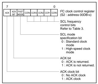
Fig. 14. Structure of I<sup>2</sup>C clock control register
