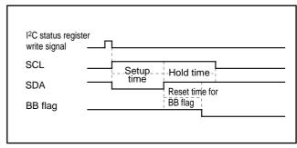
Fig. 20. STOP condition generating timing diagram
