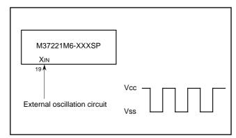
Fig. 55. External clock input circuit example
