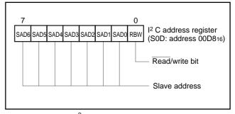
Fig. 13. Structure of I<sup>2</sup>C address register
