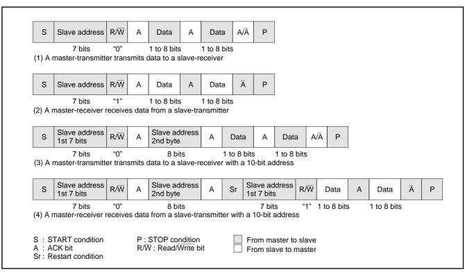
Fig. 22. Address data communication format
