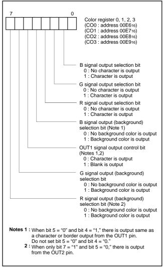
Fig. 42. Structure of color registers
