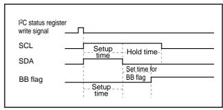
Fig. 19. START condition generating timing diagram
