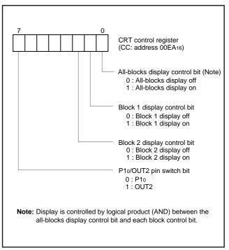
Fig. 32. Structure of CRT control register
