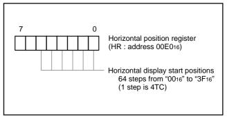
Fig. 37. Structure of horizontal position register
