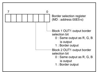
Fig. 43. Structure of border selection register
