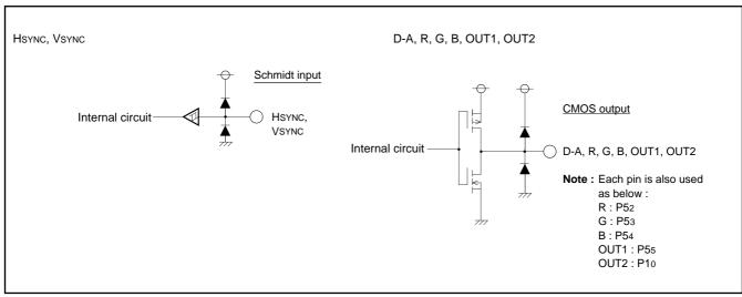
Fig. 53. I/O pin block diagram (2)
