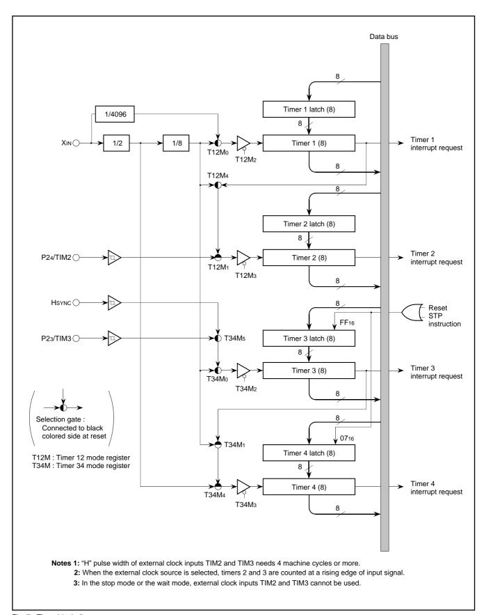
Fig. 7. Timer block diagram
