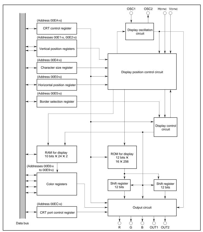
Fig. 33. Block diagram of CRT display control circuit
