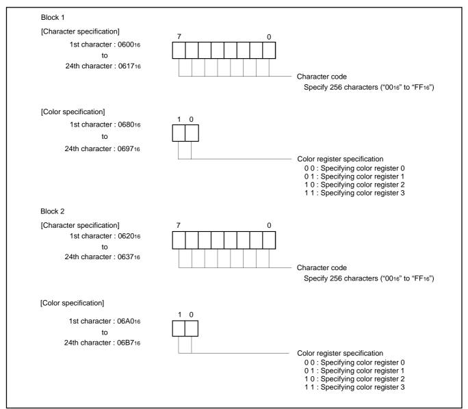
Fig. 41. Structure of CRT display RAM
