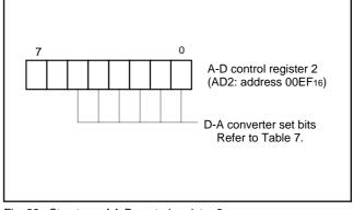
Fig. 29. Structure of A-D control register 2
