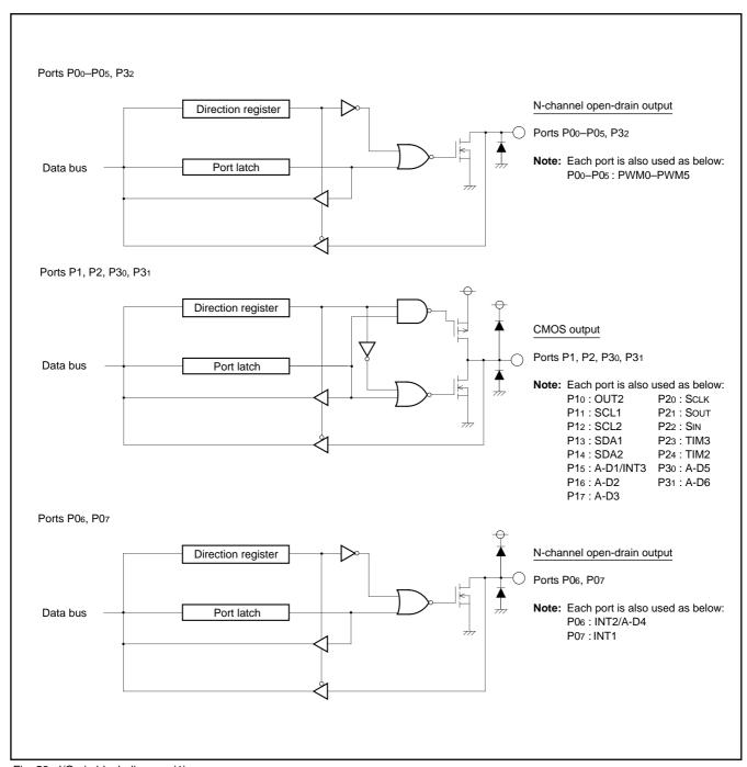
Fig. 52. I/O pin block diagram (1)
