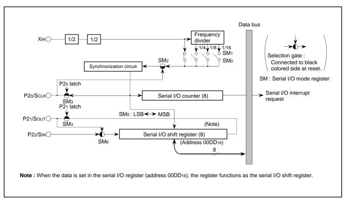
Fig. 8. Serial I/O block diagram
