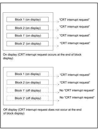
Fig. 45. Timing of CRT interrupt request
