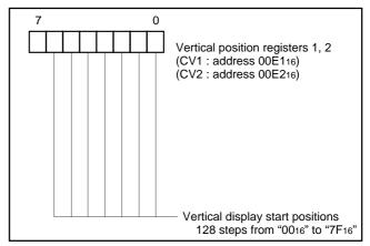
Fig. 36. Structure of vertical position register
