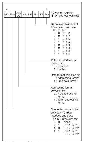
Fig. 16. Structure of I<sup>2</sup>C control register
