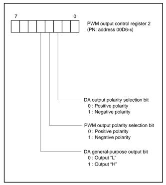
Fig. 27. Structure of PWM output control register 2
