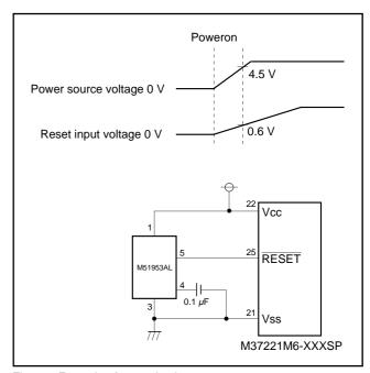
Fig. 50. Example of reset circuit
