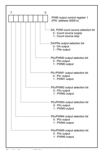
Fig. 26. Structure of PWM output control register 1
