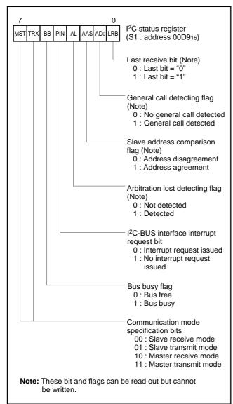
Fig. 17. Structure of I<sup>2</sup>C status register
