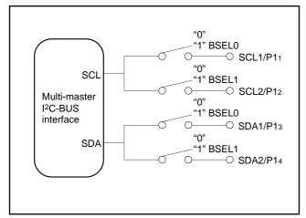
Fig. 15. Connection port control by BSEL0 and BSEL1
