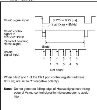
Fig. 35. Supplement explanation for display position
