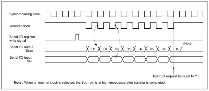
Fig. 10. Serial I/O timing (for LSB first)
