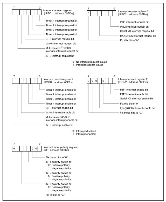
Fig. 4. Structure of interrupt-related registers
