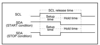
Fig. 21. START condition/STOP condition detecting timing diagram
