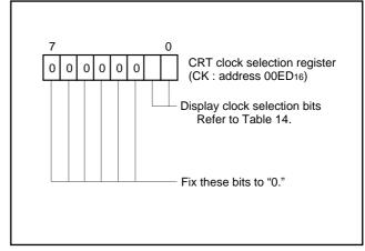
Fig. 48. Structure of CRT clock selection register
