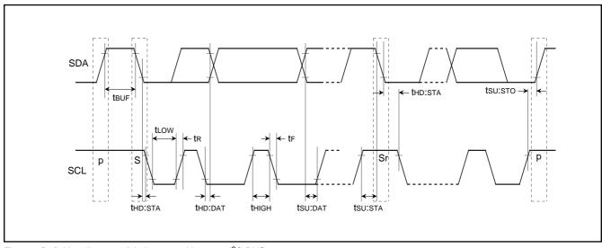
Fig. 59. Definition diagram of timing on multi-master I<sup>2</sup>C-BUS
