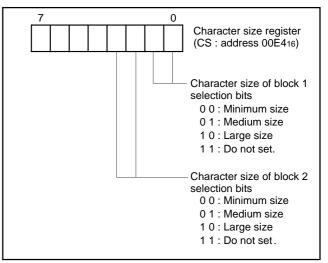
Fig. 38. Structure of character size register
