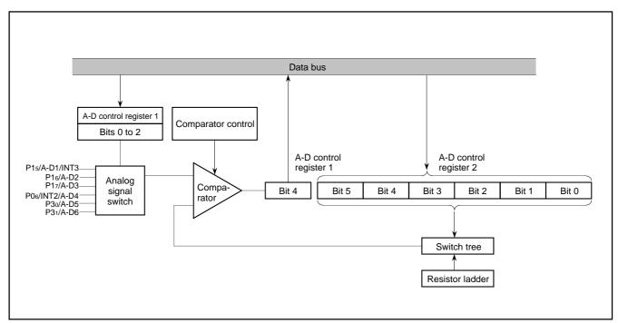
Fig. 30. A-D comparator block diagram
