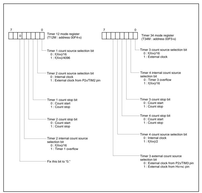
Fig. 6. Structure of timer-related registers
