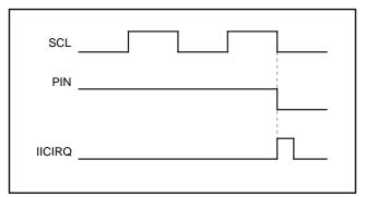
Fig. 18. Interrupt request signal generating timing
