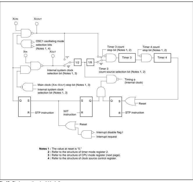
Fig. 95. Clock generating circuit block diagram
