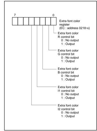
Fig. 70. Structure of extra font color register
