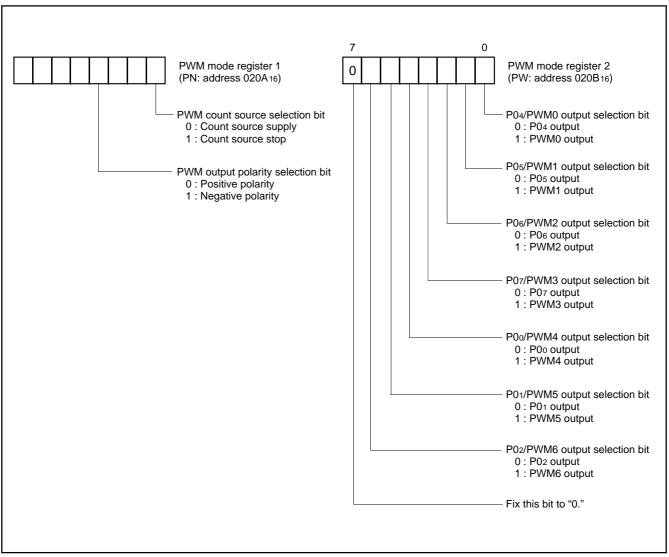
Fig. 17. Structure of PWM-related registers
