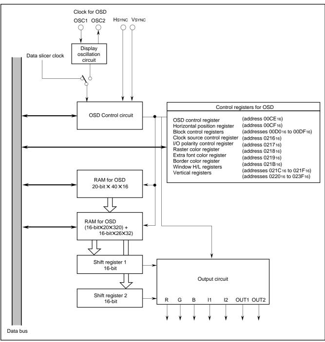
Fig. 51. Block diagram of OSD control circuit
