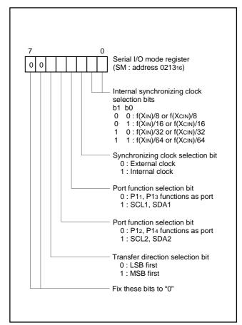
Fig. 14. Structure of serial I/O mode register
