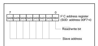
Fig. 40. Structure of I<sup>2</sup>C address register
