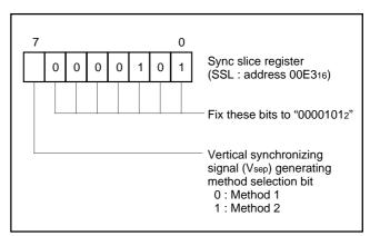
Fig. 24. Structure of sync slice register
