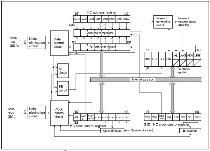
Fig. 39. Block diagram of multi-master I<sup>2</sup>C-BUS interface
