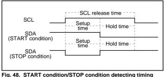
Fig. 48. START condition/STOP condition detecting timing diagram
