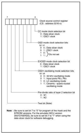
Fig. 62. Structure of clock control register
