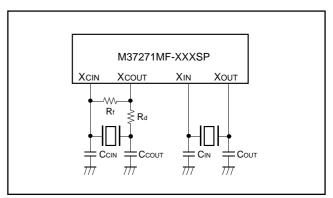
Fig. 93. Ceramic resonator circuit example
