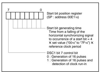
Fig. 29. Structure of start bit position register
