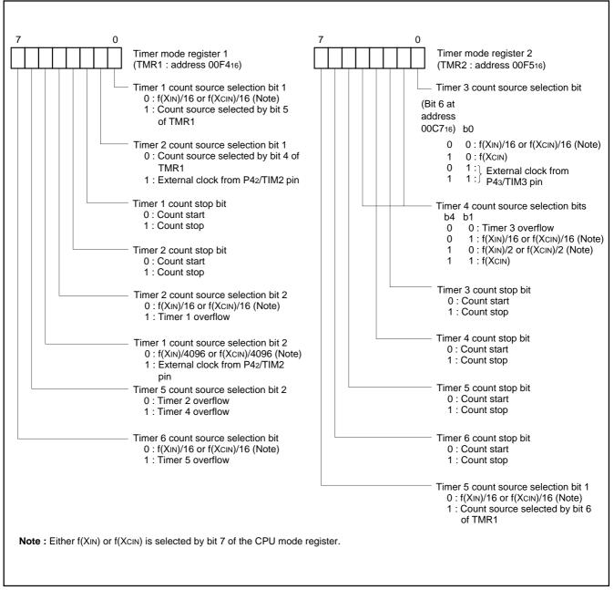
Fig. 10. Structure of timer-related registers
