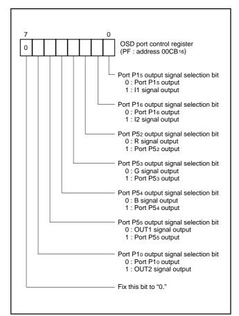
Fig. 83. Structure of OSD port control register
