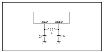
Fig. 97. Display oscillation circuit
