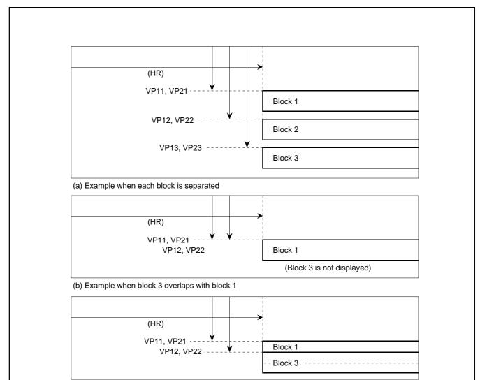
(c) Example when block 3 overlaps in process of block 1
