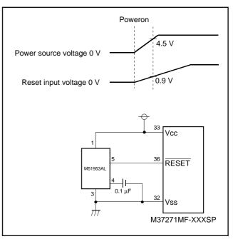
Fig. 89. Example of reset circuit
