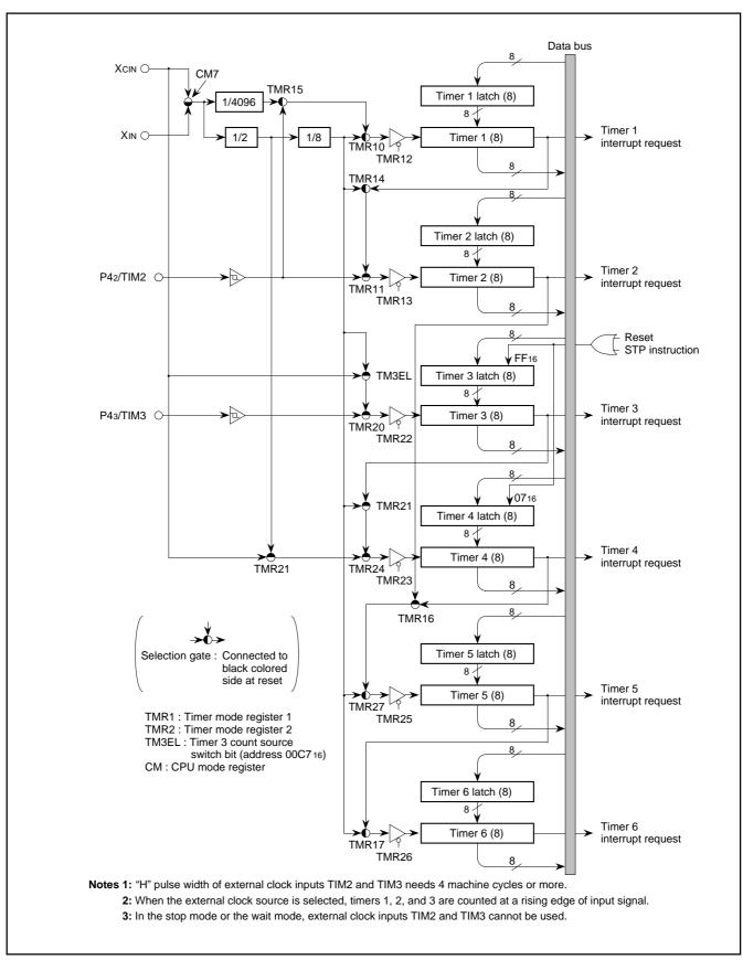
Fig. 11. Timer block diagram
