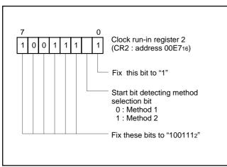
Fig. 30. Structure of clock run-in register 2
