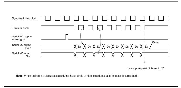
Fig. 13. Serial I/O timing (for LSB first)
