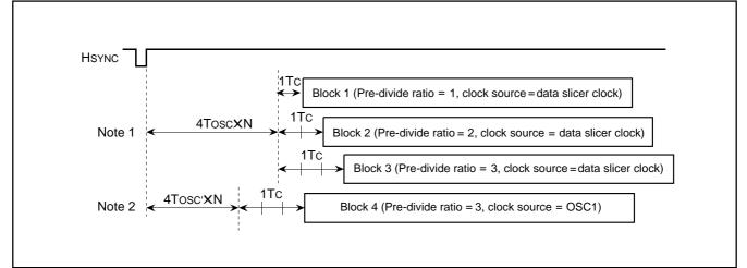
Fig. 60. Notes on horizontal display start position
