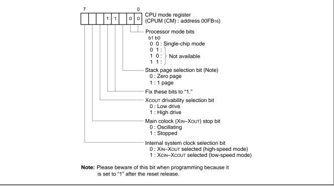
Fig. 1. Structure of CPU mode register
