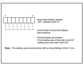
Fig. 59. Structure of horizontal position register
