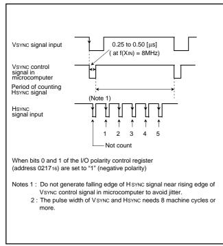
Fig. 57. Supplement explanation for display position
