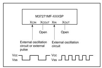
Fig. 94. External clock input circuit example
