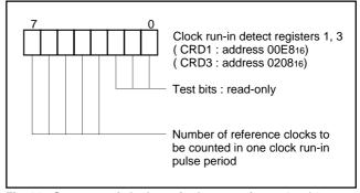
Fig. 36. Structure of clock run-in detect registers 1 and 3
