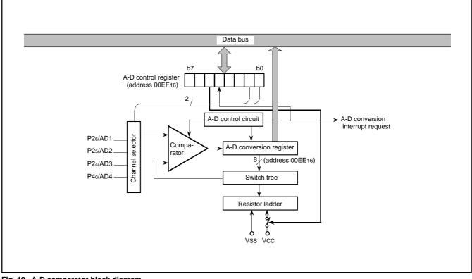
Fig. 19. A-D comparator block diagram
