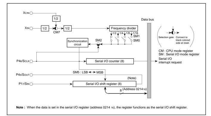
Fig. 12. Serial I/O block diagram
