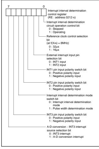
Fig. 87. Structure of interrupt interval determination control register
