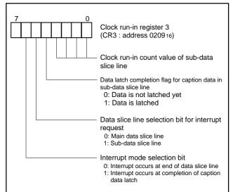
Fig. 34. Structure of clock run-in register 3
