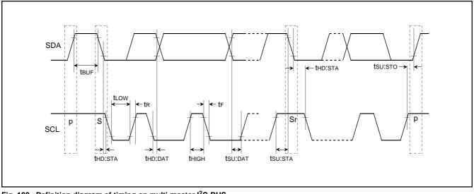
Fig. 100. Definition diagram of timing on multi-master I<sup>2</sup>C-BUS
