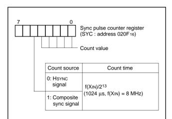
Fig. 37. Sync pulse counter register
