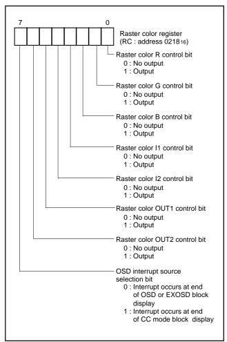
Fig. 84. Structure of raster color register
