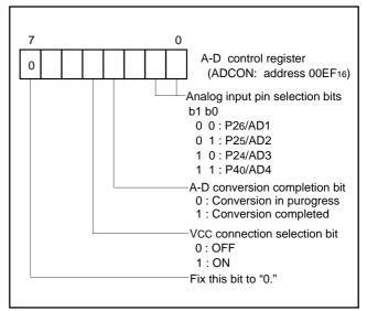
Fig. 18. Structure of A-D control register
