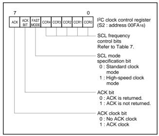
Fig. 41. Structure of I<sup>2</sup>C clock control register
