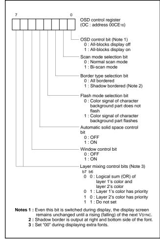
Fig. 52. Structure of OSD control register
