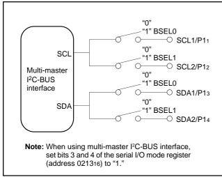
Fig. 42. Connection port control by BSEL0 and BSEL1
