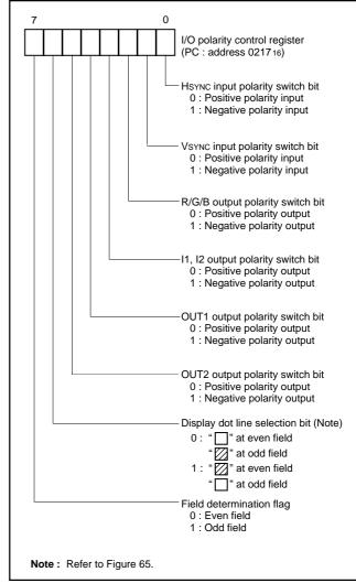
Fig. 64. Structure of I/O polarity control register
