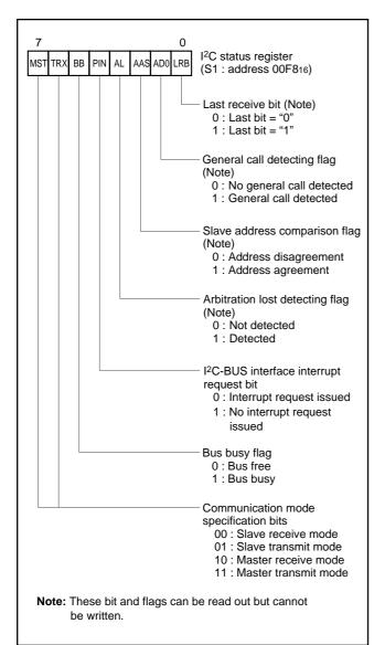
Fig. 44. Structure of I<sup>2</sup>C status register
