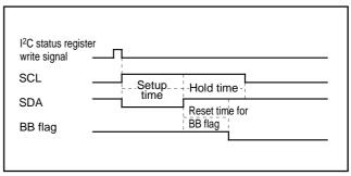
Fig. 47. STOP condition generating timing diagram
