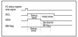
Fig. 46. START condition generating timing diagram
