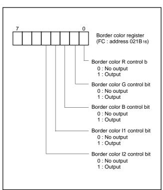
Fig. 77. Structure of border color register
