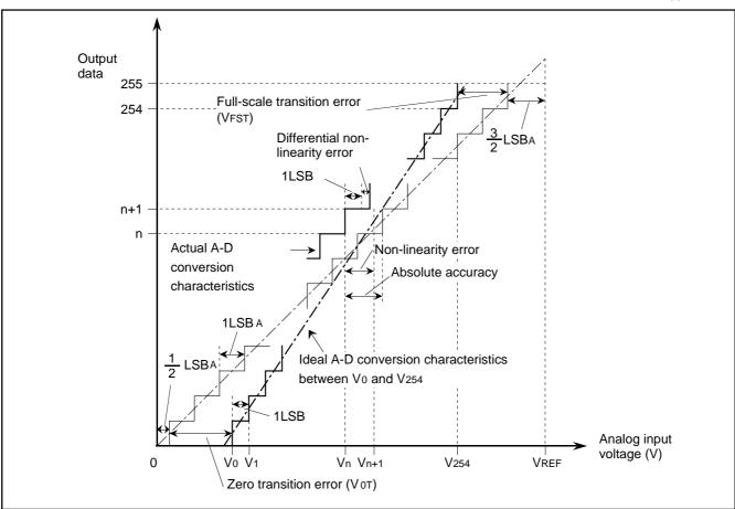
Fig. 21. Definition of A-D conversion precision
