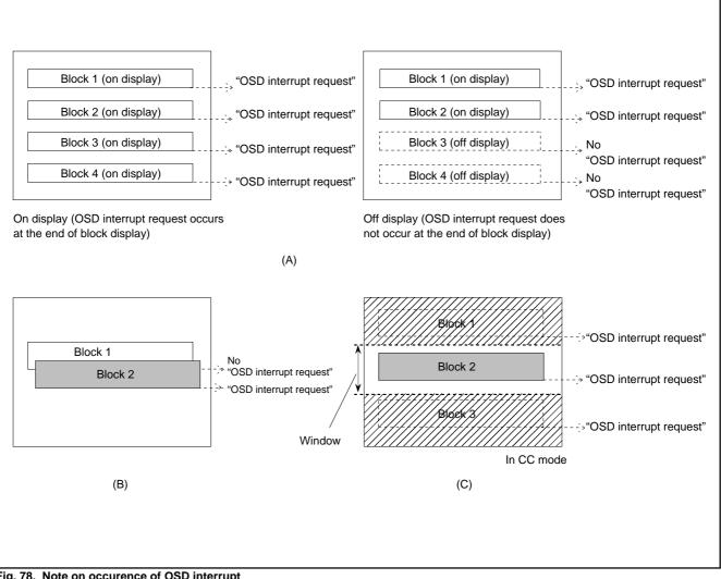
Fig. 78. Note on occurence of OSD interrupt
