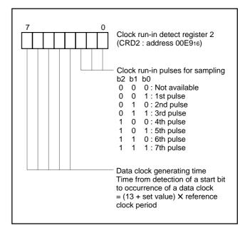
Fig. 31. Structure of clock run-in detect register 2
