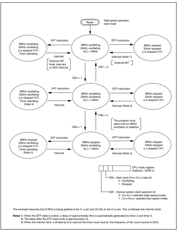
Fig. 96. State transitions of system clock
