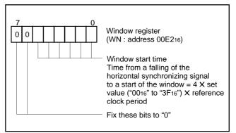
Fig. 32. Structure of window register
