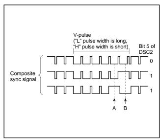
Fig. 26. Determination of V-pulse waveform
