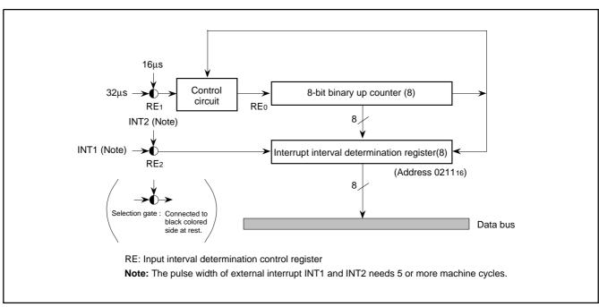
Fig. 86. Block diagram of interrupt interval determination circuit
