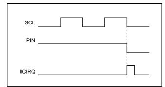
Fig. 45. Interrupt request signal generating timing
