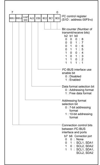
Fig. 43. Structure of I<sup>2</sup>C control register
