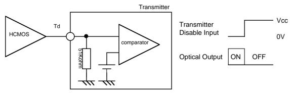
The transmitter is normally enabled and only requires an external voltage to disable.
