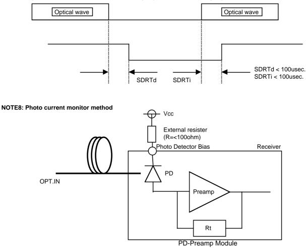
The photocurrent will be calculated based on the voltage drop across on external resistor connected between the monitoring pin and +5V.
