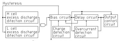
To overcharge detection circuit
