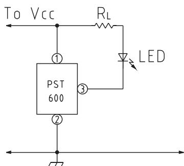
Note : When V<sub>CC</sub> line impedance is high, connect a capacitor between IC Pins 1 and 2.
