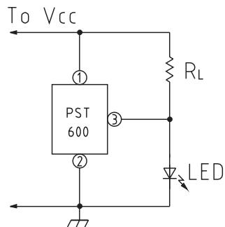
Note : When V<sub>CC</sub> line impedance is high, connect a capacitor between IC Pins 1 and 2.
