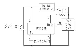
Rise delay time (T1) and No-response time (T2) using external capacitor
