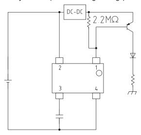
Note: When Vcc is less than LED VF, take LED lamp power from DC-DC converter or other output.
