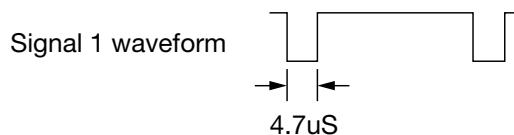
\*3 Measuring horizontal sync signal pull-in range
