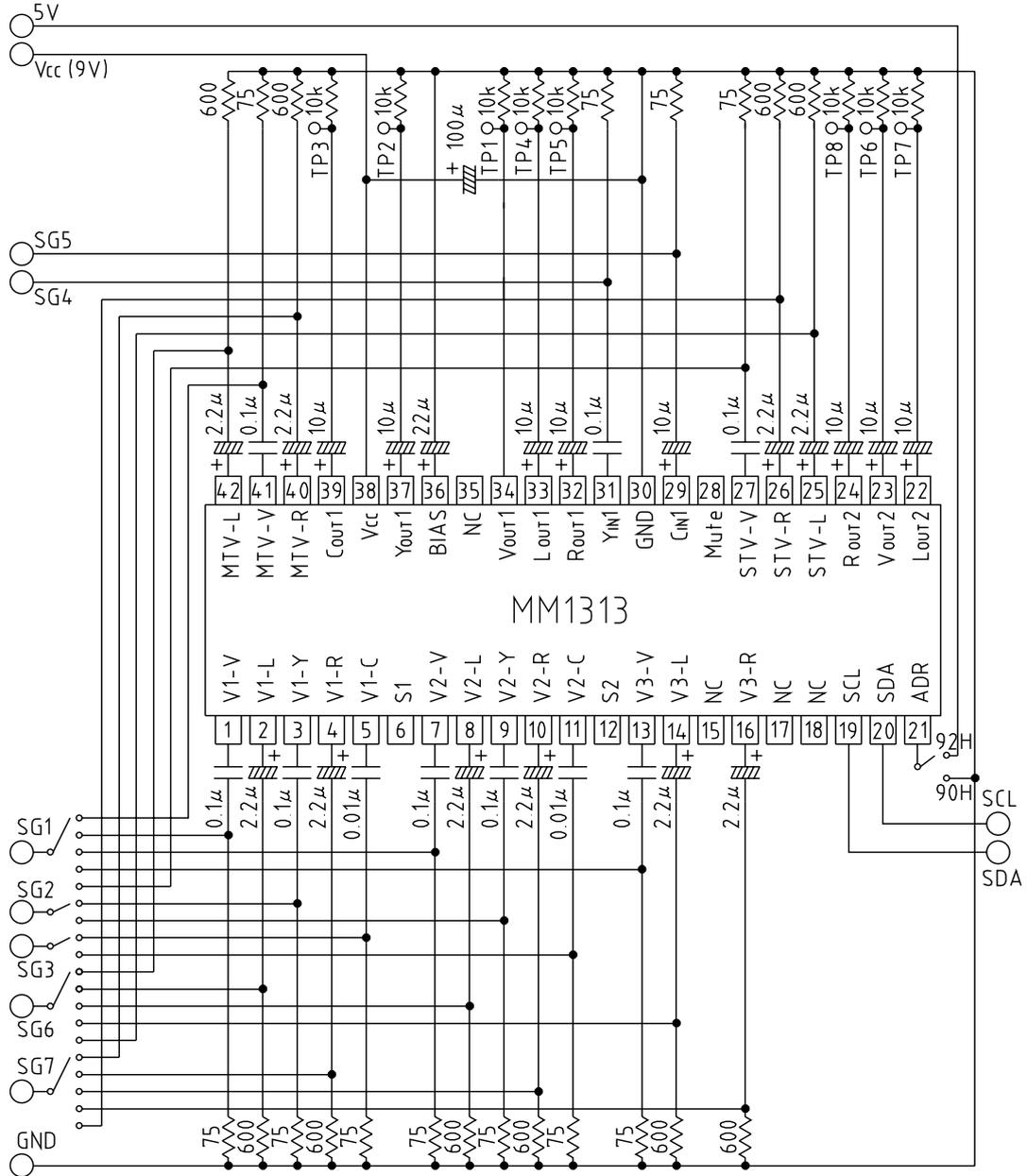
■ Measurement Circuit 2 (Crosstalk measurement)
