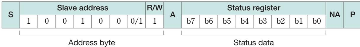
The data format is set as shown in the figure above. The first 7 bits in the address byte are allocated to the slave address, and the remaining 1 bit is allocated to the read/write bit. The read/write bit is set at 1 when using as a status register.
