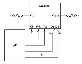
Figure 12. Typical 8-Bit µP Interface, Double Write
