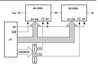
Figure 16. Operation as Logarithmic D/A Converter
