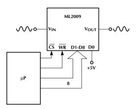
Figure 13. Typical 8-Bit µP Interface, Single Write
