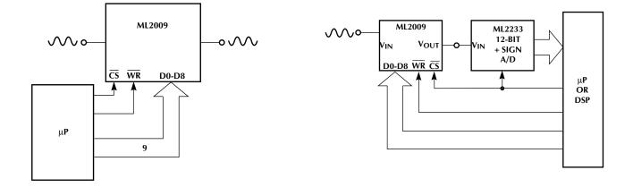
Figure 14. Typical 16-Bit µP Interface Figure 15. AGC for DSP or Modem Front End
